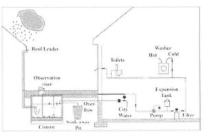
FIGURE 5-14 Rainwater harvesting tanks at a Starbucks in Austin, Texas. SOURCE: Laura Ehlers.
